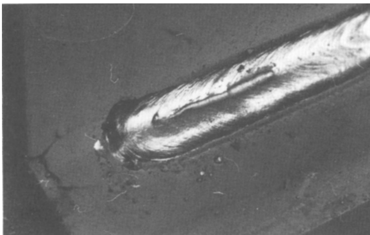
4.2 Gas trails on the surface of a weld made with rutile flux-cored wire.
