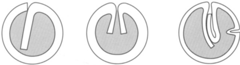
2.7 Tubular wires with folded sections.
